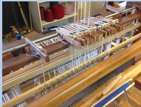
Loom modification for shaft switching
